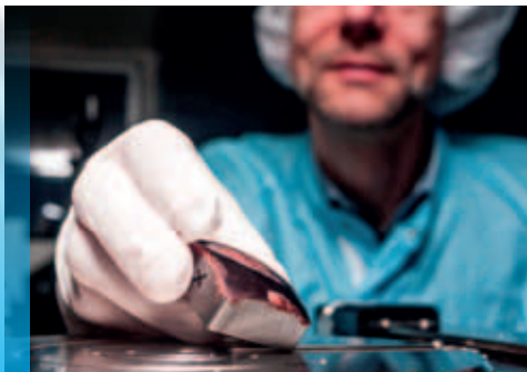
A doubly curved stamp produced by Nil Technologies A/S is characterized by Atomic Force Microscopy at DFM
