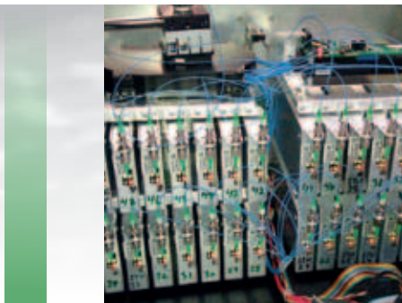
The picture shows a multi-channel laser system being prepared for shipment. The system includes 28 individual laser modules of the new frequency stabilized design.
