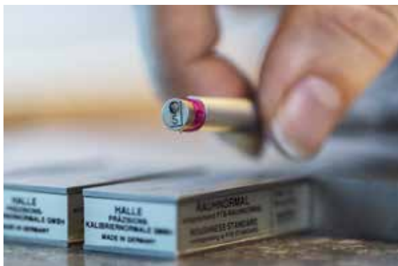
Positioning of the stylus onto a roughness standard.
