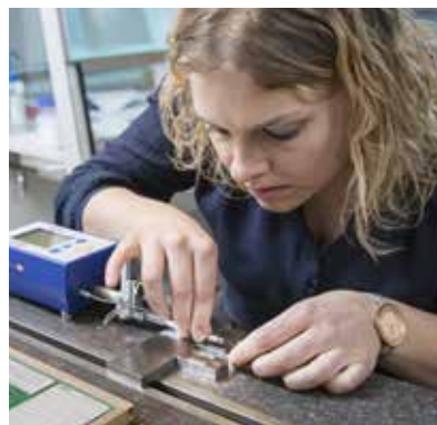
Calibration of a hand held roughness tester against roughness standards of different roughness levels.
