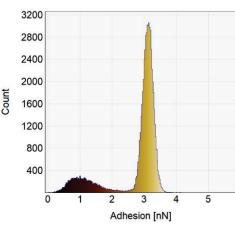
Example: The figure on the left shows an adhesion map of a two-component polymer blend (PS-LDPE) measured with AFM. The figure on the right shows a histogram illustrating the difference between adhesion forces of the two components.
